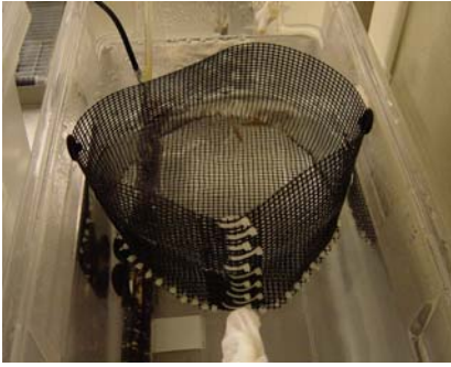
Figure 1: Spawning tank. A 5 gallon flow-trough tank is fitted with a mesh cage that holds broodstock.
